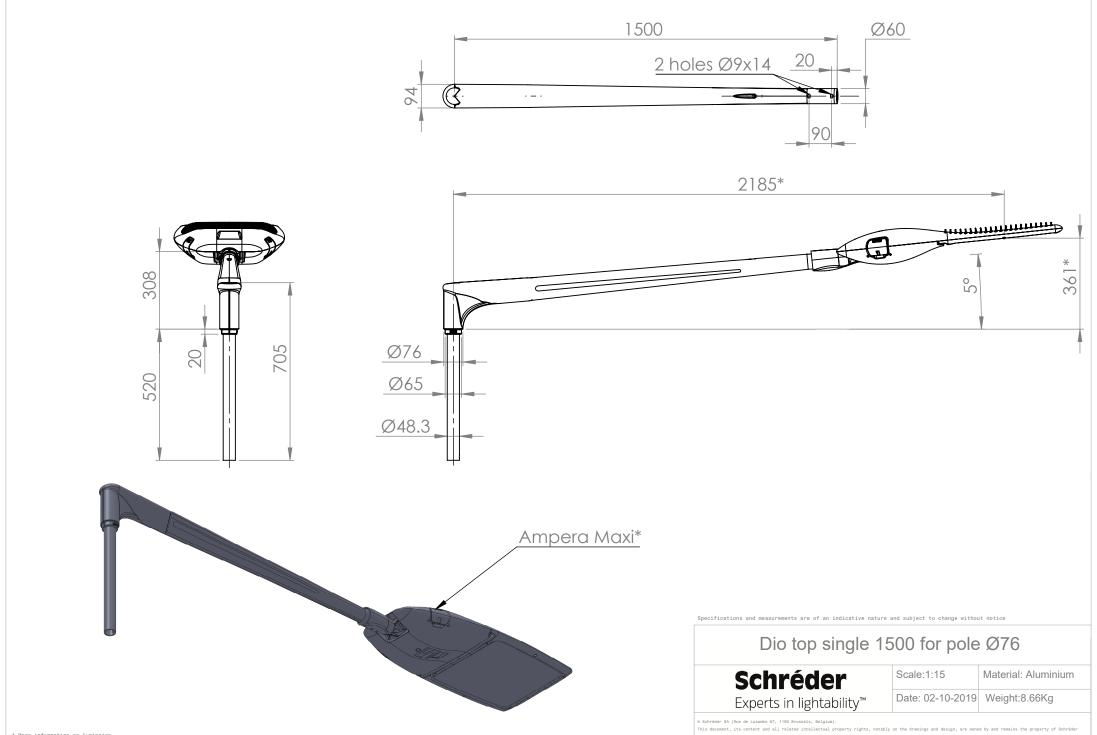
\* More information on luminaire compatibility is available in the datasheet This document, its content and all related intellectual property rights, notably on the drawings and design, are owned by and remains the property of Schröder SA. In no case, it can be used for unauthorized purposes. It can not be reproduced or communicated to third parties without Schröder's express and written agreement. Infringement gives rights to damages.
