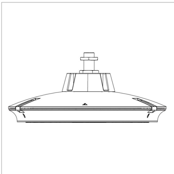
FLEXIA FG | Suspensa penetrada 1" gas (S3)
